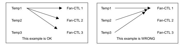
Any temperature monitor can be used for all of the reference for the fan control.
